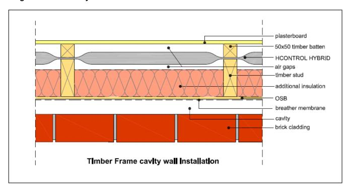
Figure 7: Two Layers of HControl Hybrid on Timber Frame Wall
