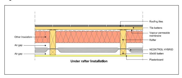
Figure 4: Installation under Rafters without Battens
