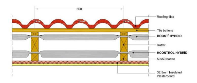
Roof 4: 600mm rafter spacing - Non ventilated pitched roof BOOST'R HYBRID HCONTROL HYBRID 32.5mm INSULATED PLASTERBOARD U-VALUE = 0.18 W/m²K
