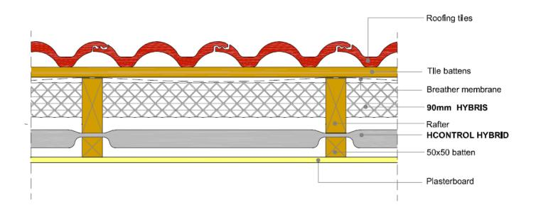
Roof 7: 600mm rafter spacing - Non ventilated pitched roof 90mm HYBRIS HCONTROL HYBRID U-VALUE = 0.18 W/m²K
