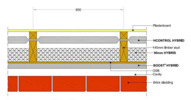
Timber frame wall 7: 140mm timber stud BOOST'R HYBRID 90mm HYBRIS HCONTROL HYBRID U-VALUE = 0.14 W/m²K
