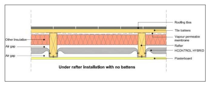
Figure 5: Two Layer Insulation
